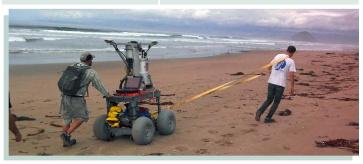
CSU Monterey Bay-CSU Fresno team mapping the Morro Bay sand spit using a terrestrial laser scanner. Image courtesy of Dr. Rikk Kvitek, CSUMB.
