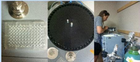
Farthest left shows samples wrapped in small tins for analysis. Each row includes soil samples from treatment pond one and four. The center picture shows how samples are loaded into the auto analyzer. On the right samples are loaded into place to be analyzed.
