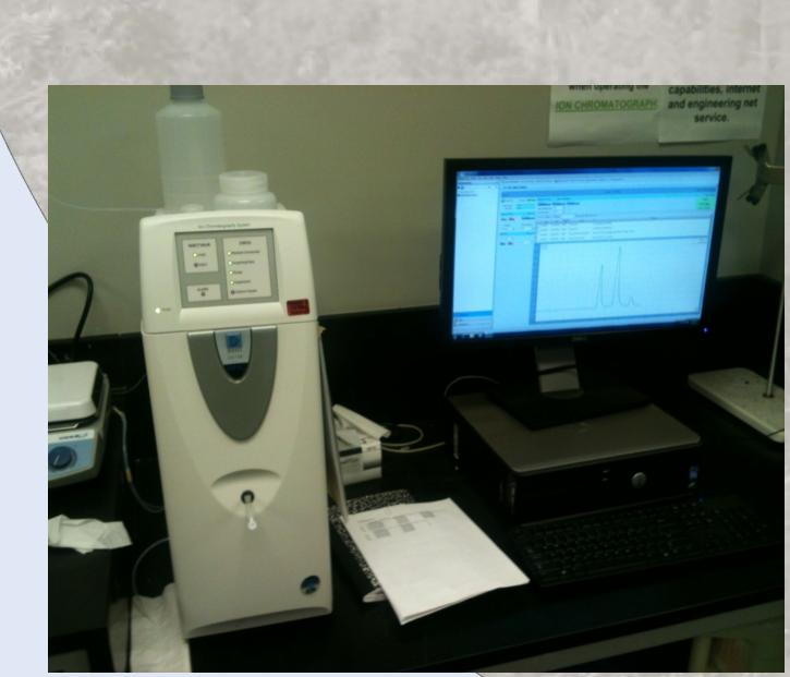
Figure 4: Ion Chromatograph used to analyze the concentration of nitrate in the influent and effluent.
