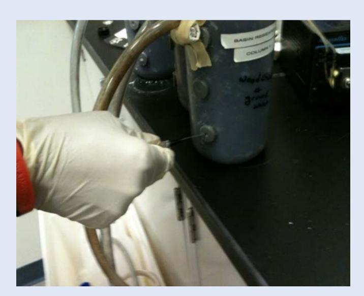
Figure 3: Injection of succinate through the use of rubber ports positioned 1inch apart along the length of the column
