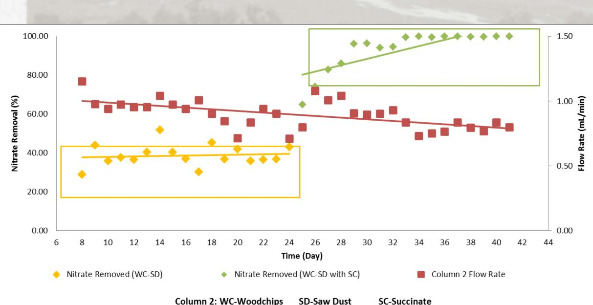
Figure 6: Woodchips and sawdust system results. Nitrate Removed (%) and Flow Rate (mL/min) vs Time (Days); The flow rate was maintained at a constant 1.0 mL/min throughout the project. Days 8-24 (without succinate indicated by the yellow square) show a nitrate removal of percent 38%; Days 25-41 show (with succinate indicated by the green square) show a nitrate removal of 93%.
