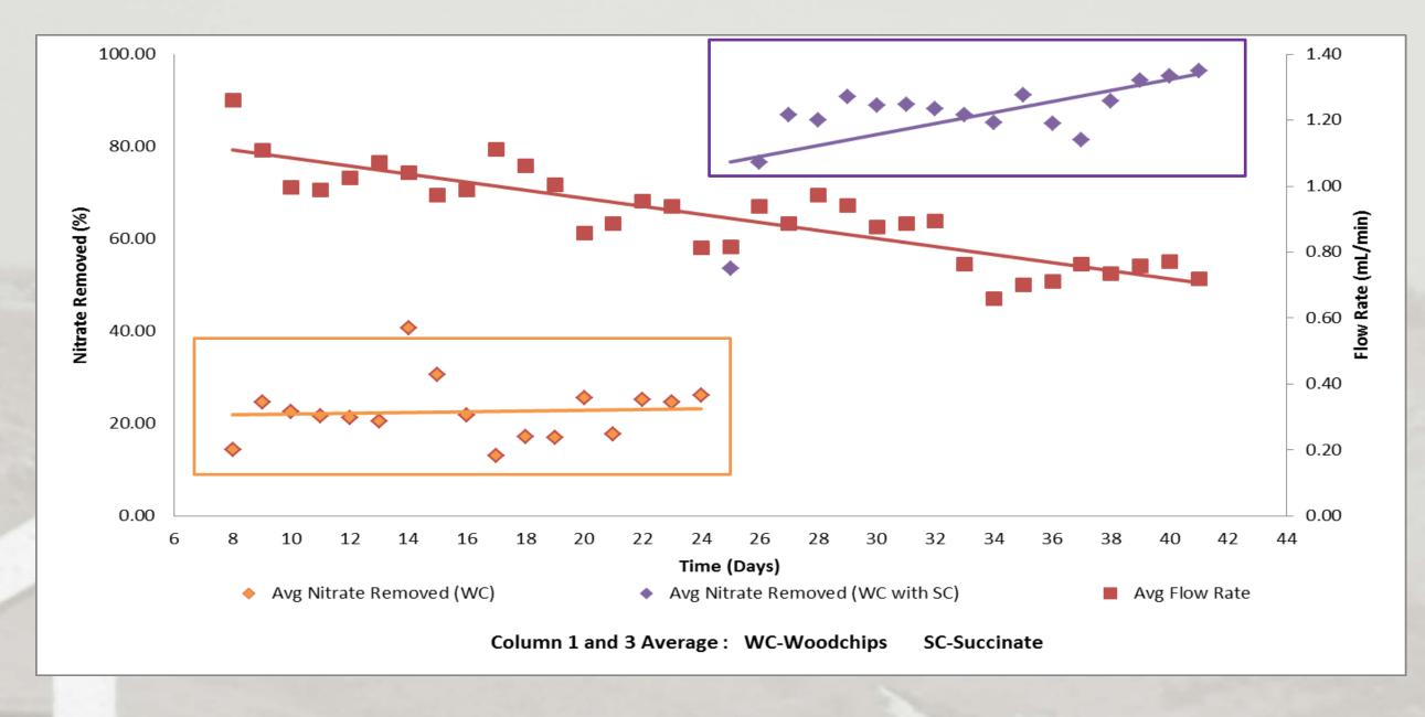
Figure 5: The average of the woodchip system results. Nitrate Removed (%) and Flow Rate (mL/min) vs Time (Days); The average flow rate of the two systems was maintained at a constant 1.0 mL/min. Days 8-24 (without succinate indicated by an orange square) show a nitrate removal of percent 23%; Days 25-41 show (with succinate indicated by a purple square) show a nitrate removal of 86%.
