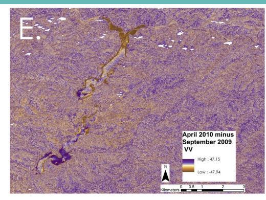
Change detection between a wet period (April 2010) and a dry period (Sept 2009) for different UAVSAR polarizations. Image **C** shows change in soil moisture and image **D** highlights changes in water; positive values indicate more moisture in April 2010. Image **E** shows changes in vegetation with positive values indicating more vegetation in April 2010.
