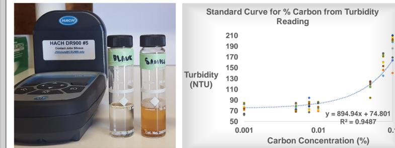
Fig 7. Left: Sample cells used in HACH Colorimeters for NO<sub>3</sub><sup>-</sup> readings. Right: Standard curve allows carbon concentration to be calculated from turbidity.
