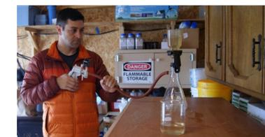
Fig 8. Hand pump filtration device used to separate particles from sample water.
