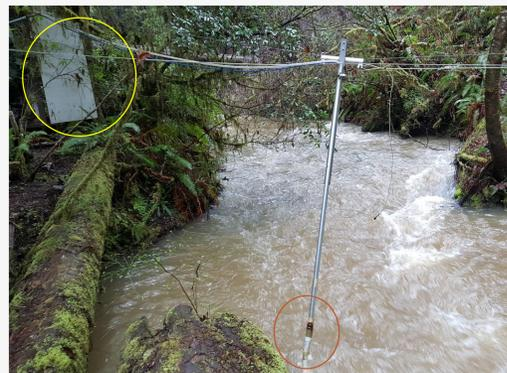
Figure 2: The gauge site during a high flow event. The turbidity probe is circled in orange and the station containing the equipment is circled in yellow.
