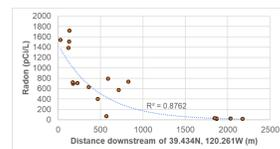
Graph showing radon activity levels at points along Sagehen Creek (Moran et al. 2022). Radon levels decrease more or less exponentially down the reach of the stream that was sampled, suggesting that the highest groundwater discharge to the creek is found within Kiln Meadow and that there is less groundwater discharge to the creek further downstream.
