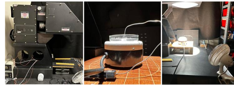
Figure 4. Solar simulator experimental setup with fan for temperature stability
