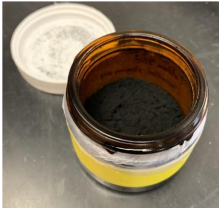
Pristine, cryomilled tire tread particles 32.2 \mu\text{m} \pm 25.5 \mu\text{m}
